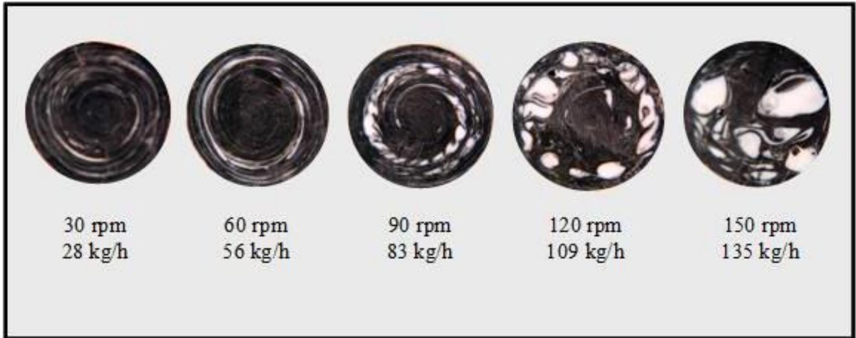
Cross-sectional views of extrudate samples at a letdown ratio of 100 to 1 of a white pigmented ABS resin with a black color concentrate for a melting-mixing experiment.
